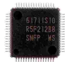
64pin LQFP 14 x 14 x 1.7mm 0.8mm pitch
